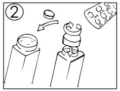
2. Add 1 pH TesTab in the vial, screw the cap.
