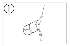
1. Submerge the small glass vial into the water collection bucket. Carefully remove the vial from the water sample, keeping the vial full to the top.
