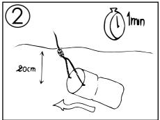
2. Throw the collection bucket in the water without twist the wire. TIP: Hold the top part strongly so that the bucket doesn't slip away from your hands during the launch. Once it's in the water, allow the water to flow into the bucket for 30 seconds while it is still submerged (about 20 cm under the surface).
