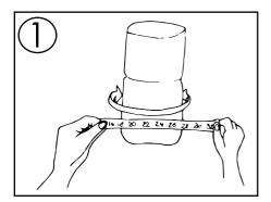
1. Adhere a thermometer strips on the outside bottom of your collector bucket.
