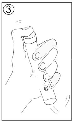
3. Cap and mix until the tablet has completely dissolved. Bits of material may remain in the sample.
