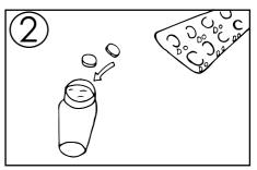
2. Drop two Dissolved Oxygen TesTabs into the vial. Water will overflow when the tablets are added.
