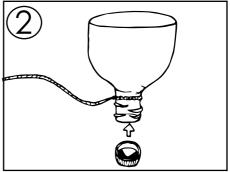
2. Screw the cap inside the second part of the collector bucket (top part of the bottle)
