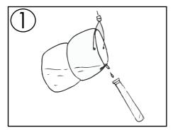
1. Fill the test tube until the 10 ml line with the water sample
