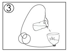
3. Pour out some water sample inside the top part of the bucket collector sample.
