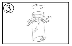
3. Screw the cap on the vial. More water will overflow as the cap is tightened. Make sure no bubbles are present in the sample.
