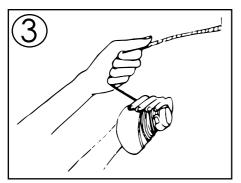
3. Rewind the wire back while using the top part of the bucket for keeping the wire together.
