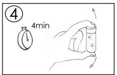
4. Mix by inverting the vial over and over until the tablets have dissolved. This will take about 4 minutes.
