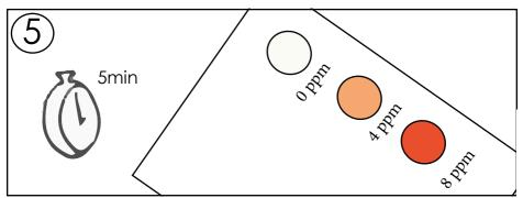
5. Wait 5 more minutes for the color to develop. Clock . Compare the color of the sample to the color comparison chart. Record the result as ppm dissolved oxygen.
