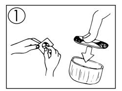
1. Remove the Turbidity disk sticker and adhere on the inner side of a cap
