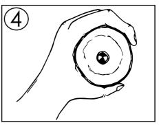
4. Check now the Turbidity by looing down to the adhesive at the bottom of the bottle.
